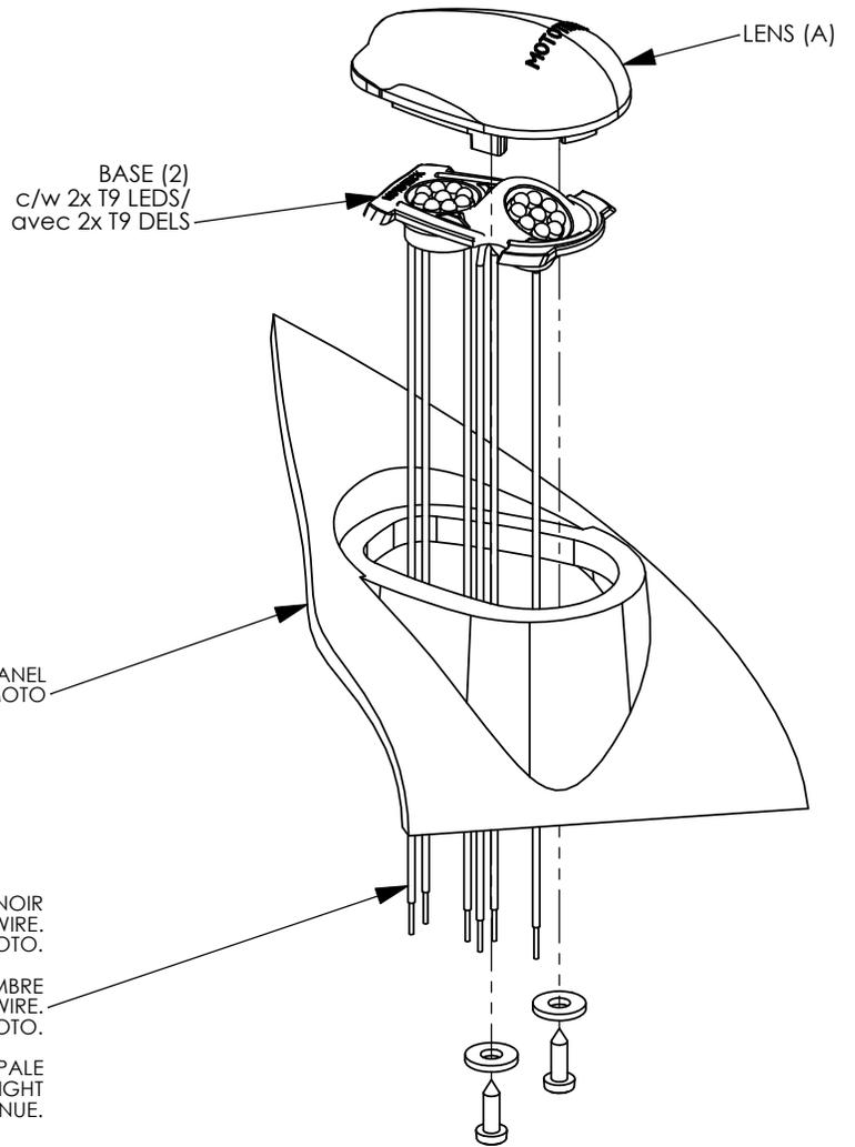
We recommend that you pre-form the threads (all the way) with the supplied screws before installation. This way you can use a 1/4" wrench to install the flashers, because on some models you may not be able to use a screwdriver.
