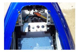
You might want to loosen or take out your tail light as it may be easier to install the undetail. Slide your rear cowl onto the bike and then slide your undertail underneath the bottom of your cowl so it slips right below your
